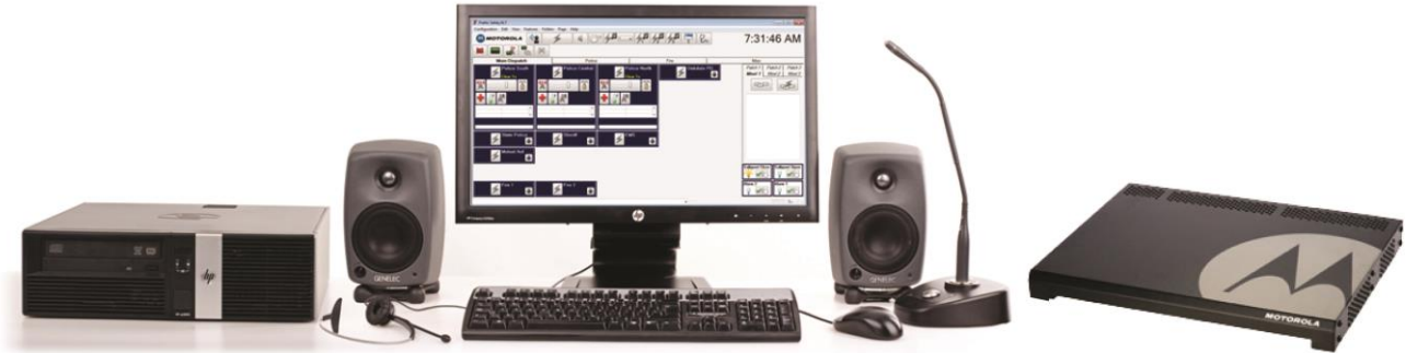
Figure 2-2: MCC 7500 Operator Position
